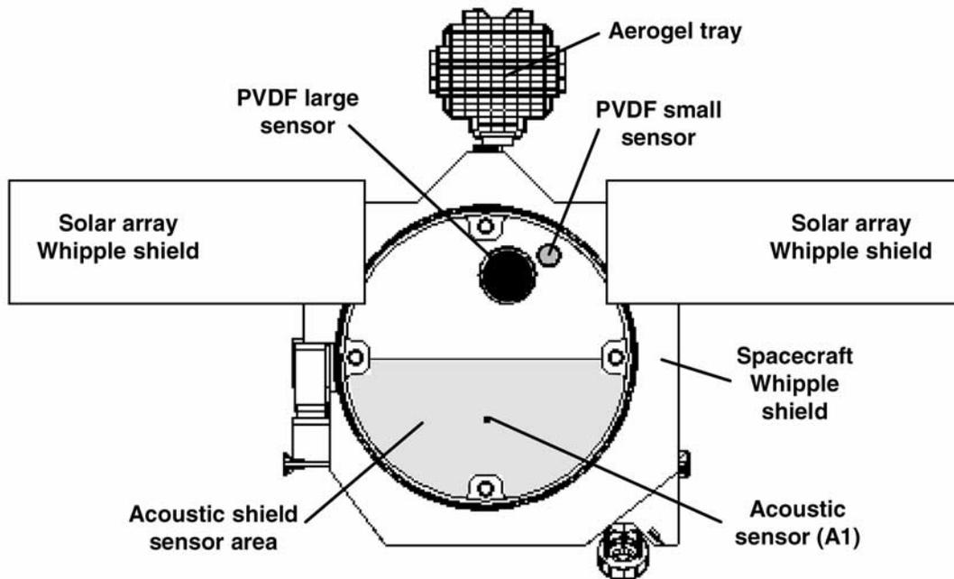
**Figure 1.** View of the Stardust spacecraft along the relative velocity vector during 81P/Wild 2 flyby, indicating the relative areas of active and inactive surfaces exposed to cometary dust impacts. The sensitive areas of the DFMI sensors are shaded. The acoustic sensor, located on the rear shield (A2), is directly behind the A1 sensor.
