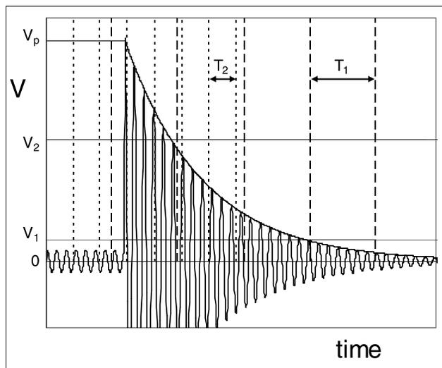
**Figure 2.** Schematic of the DFMI acoustic sensor output for counts resulting in  $N_1 = 3$  and  $N_2 = 3$  (see text for details).
