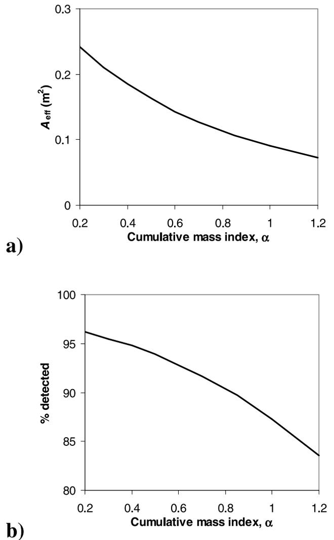
**Figure 5.** (a) The variation of effective area of the acoustic detector on the front shield as a function of cumulative mass index of the impacting particles. (b) The fraction of detected particles which are larger than the defined mass threshold of  $3 \times 10^{-11}$  kg (see text for details).
