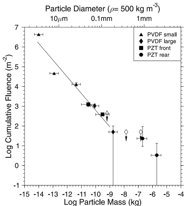
**Figure 7.** The cumulative mass distribution along the trajectory of Stardust for the entire Wild 2 encounter. Open symbols with downward arrows indicate upper limits that correspond to one impact. The solid line is the best fit mass distribution ( $\alpha = 0.85$ ) for  $m < 10^{-9}$  kg. On the upper axis the particle size is indicated assuming a density of  $500 \text{ kg m}^{-3}$ . This is for illustrative purposes only as the true density is unknown and may vary with mass.
