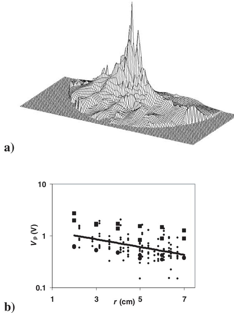
**Figure 4.** (a) Relative sensitivity of the acoustic sensor output as a function of position on the Stardust front shield. (b) Response as a function of distance  $r$  from the sensor. The large squares and circles are for data parallel and perpendicular to the straight edge of the hemispherical shield section (and passing through the sensor location).
