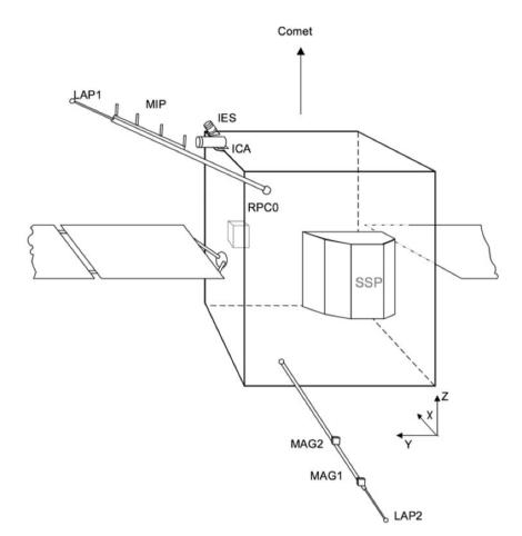
**Figure 1.** The mounting of the LAP sensors, LAP1 and LAP2, and other RPC units on the Rosetta spacecraft. RPC-0 is the common electronics box, also housing the LAP electronics boards. The direction of the s/c coordinate axes are indicated: the origin of the s/c coordinate system is at the center of the –Z surface (bottom surface in this sketch). SSP is the Philae lander, not part of RPC. [From RD13].
