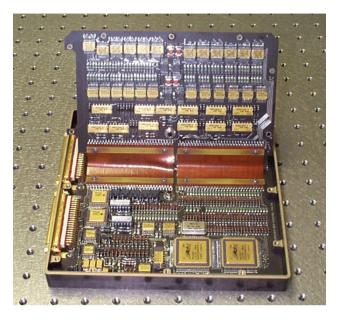
Figure 28. The Mechanism Controller Board.
