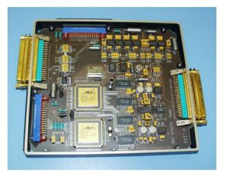
Figure 23. The CCD Readout Board.
