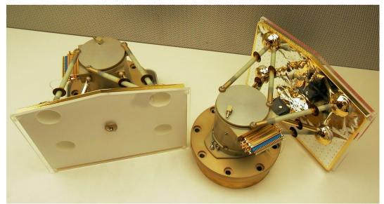
Figure 25. NAC and WAC Focal Plane Assembly.
