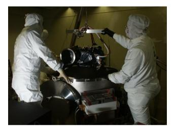
Figure 36. OSIRIS in ground calibration.
