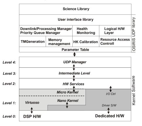
Figure 32. Structure of the OSIRIS flight software.
