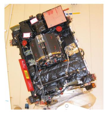
*Figure 1*. The two OSIRIS cameras (top left) with VIRTIS and the Philae lander mounted on the –x panel of Rosetta.
