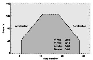
Figure 29. Nominal ramping of the motor step frequency.
