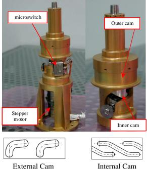
Figure 19. Components of the FDM and cylindrical development of the cams.
