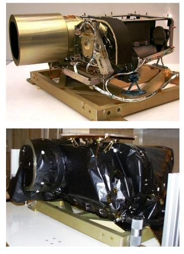
Figure 9. NAC Flight Model during integration and in flight configuration.
