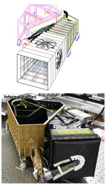
Figure 14. Concept and view of the WAC baffle.
