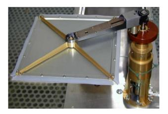
Figure 21. The integrated Front Door Mechanism.
