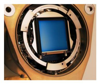
Figure 24. FPA front view with the CCD in blue colour.
