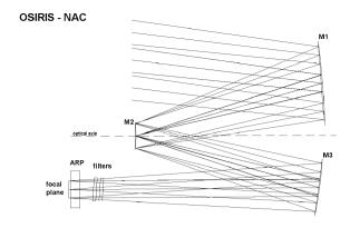
Figure 6. Ray paths through the NAC optical system.
