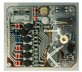
Figure 31. Power Converter Module for the CCD Readout Board.
