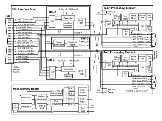
Figure 26. Block diagram of the OSIRIS DPU architecture.
