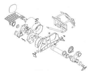
*Figure 8.* The NAC assembly. Focal plane and front door are on the upper left, primary and tertiary mirrors on the lower right.
