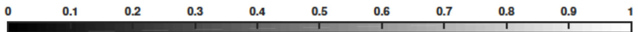
Figure 2.15: Colourscale for the illumination and the corresponding value of the cosine of the angle between the normal of the facet and the sun direction. For the FIT file, the intensity of one pixel is coded over 8 bytes, i.e., the values are between 0 and 255 in decimal basis. In order to retrieve the corresponding cosine, the value in the FIT file has to be divided by 255.
