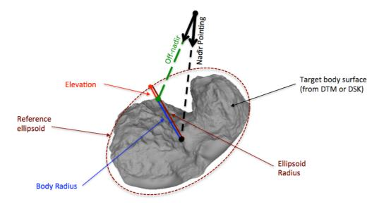
Figure 2: Observations intercepting the surface (for planets, the reference ellipsoid is in general inside the DTM)
