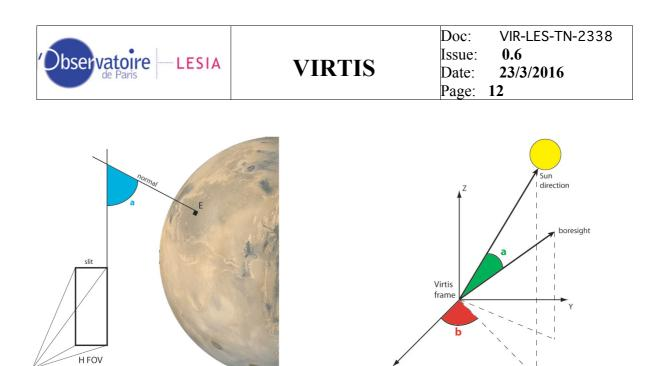
Figure 3: Slit orientation for Virtis-H
