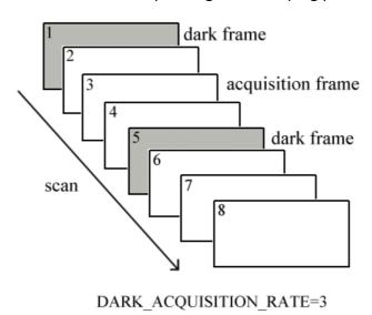
Figure 4-2: Structure of dark frames acquisition.
