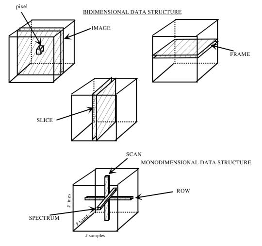
Figure 4-1: Structure of the qube data
