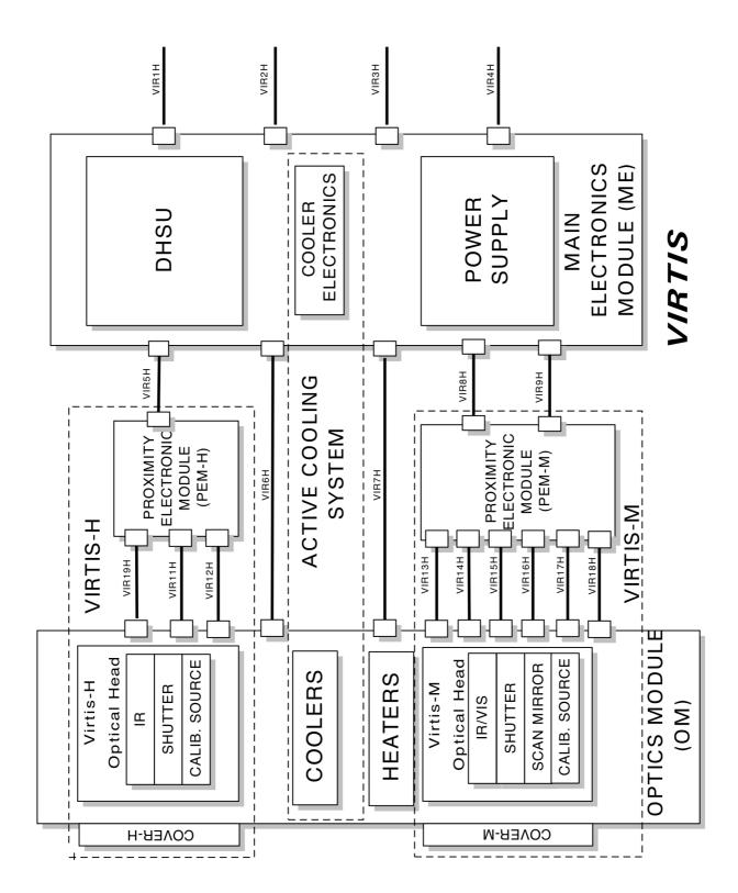
Figure 2-1:VIRTIS functional block diagram.
