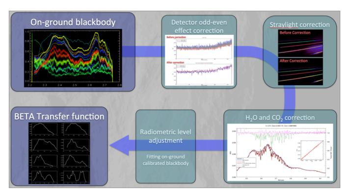
Figure 13: Flow diagram of the BETA Transfer Function creation
