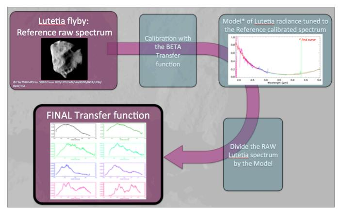
Figure 14: Flow diagram of the Final Transfer Function creation
