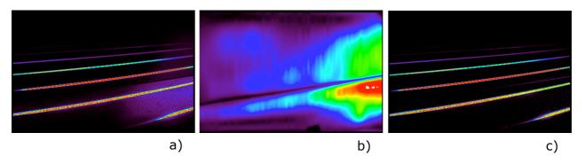
Figure 11: a) Backup raw image (2D) - b) map of the stray light - c) Backup raw image corrected from the stray light effect
