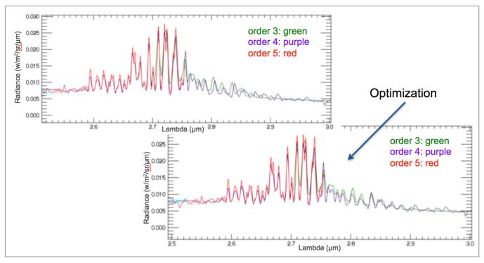
Figure 5: Optimization of the spectral registration in order 4, using ESCORT phase data and theoretical model
