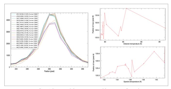
Figure 4: Registration drift estimation in spectral direction using all internal calibrations since Steins Flyby
