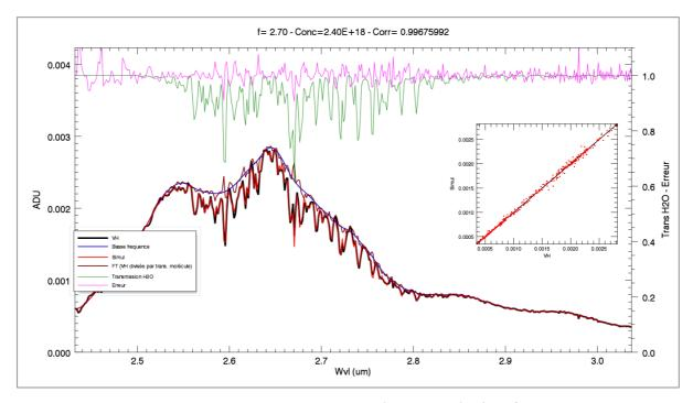
Figure 12: H2O vapor correction by HITRAN database fitting
