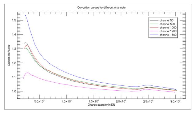
Figure 10: YACADIRE correction curve
