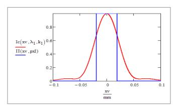
Figure 7: Spectral response @2µm, order 0
