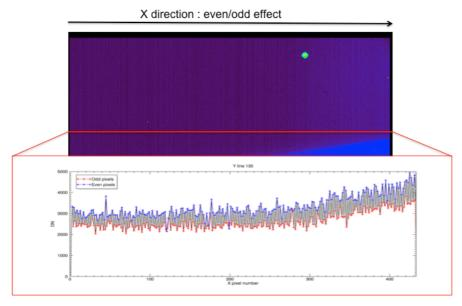
Figure 9: Odd/even effect on the Virtis-H matrix detector (Up: Backup image, Down: extraction of a pixel values in X direction)
