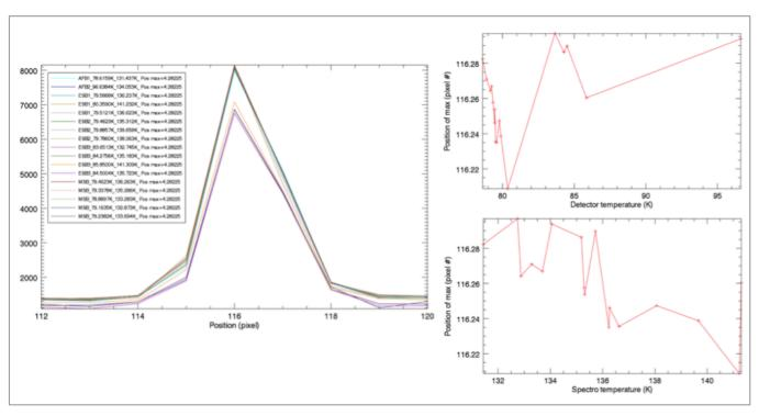
Figure 3: Registration drift estimation in spatial direction using all internal calibrations since Steins Flyby
