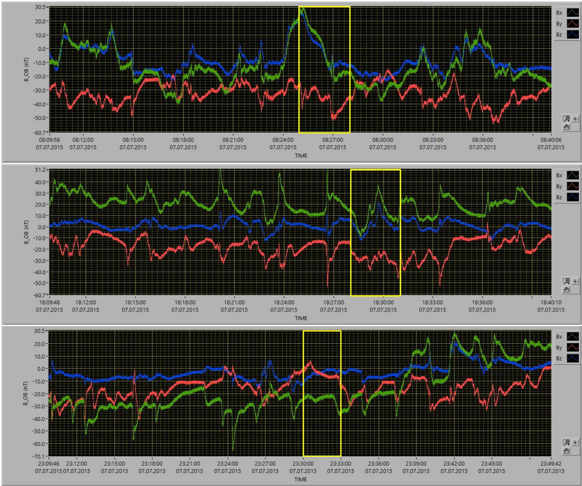
Figure 2: Examples of not visible WOL interference recorded on 07.07.2015 (top, center, bottom) during the ESC3 phase with the OB sensor. The x-axis shows time, the y-axis shows magnetic field components. Note that the scaling varies from panel to panel.
