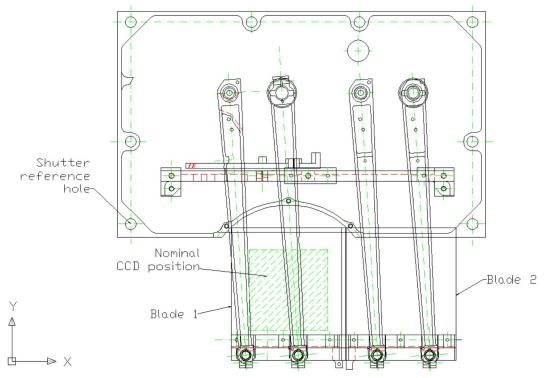
Figure 1 Shutter mechanism
