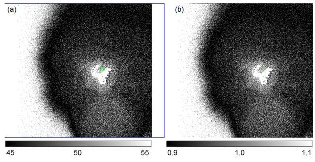
Figure 6 Ratio of single exposed and 50 exposure stacked images in level 1 (left, a) and level 2 (right, b). Values that are in the level 1 image of the single exposure below the BIAS value  $\pm$  50 DN are masked, as well as values in the non-linear regime (DN > 45000). The region of interest is shown in green.
