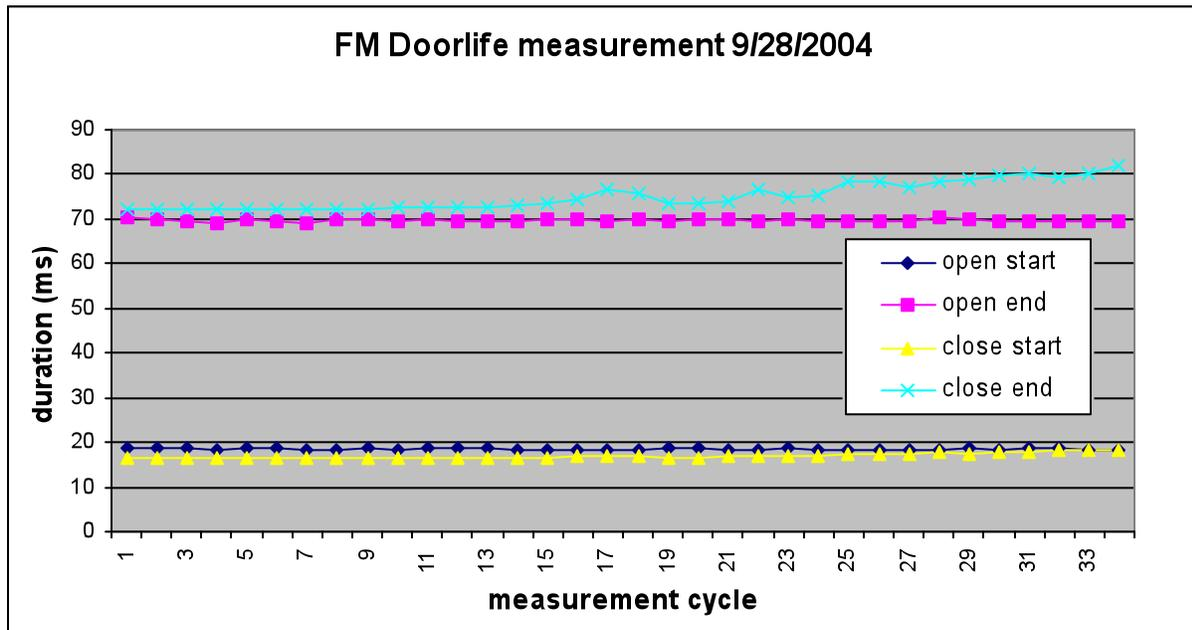
As part of the investigation into the observed trends a similar measurement was performed on the Software Test Bed (STB). The STB includes a door simulator that consists of an identical motor and two
