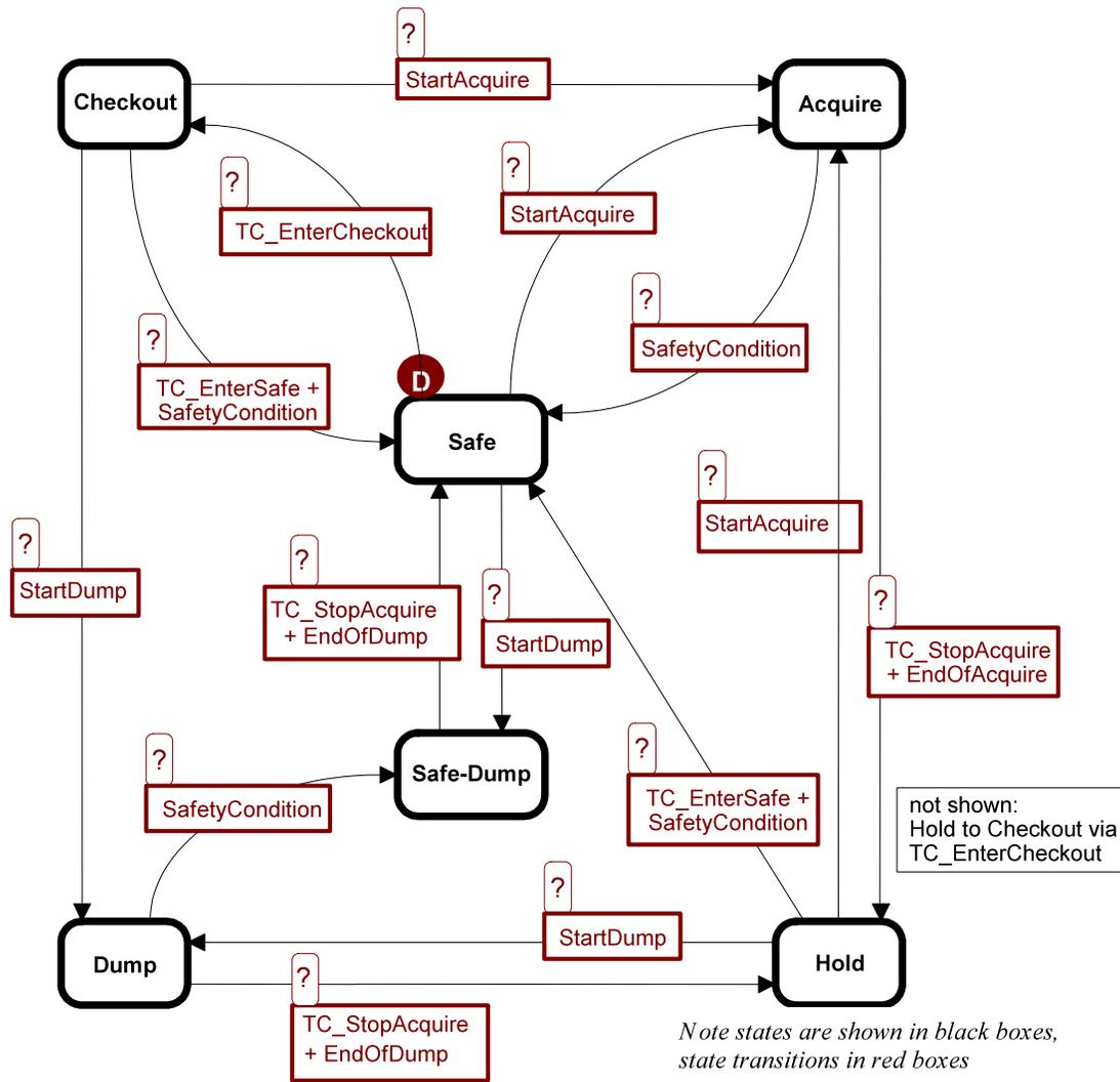
Figure 2.3-2. The Alice software operating state diagram.
