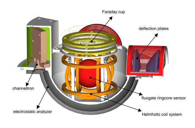
Figure 2 ROMAP MAG and SPM sensors compartment.
