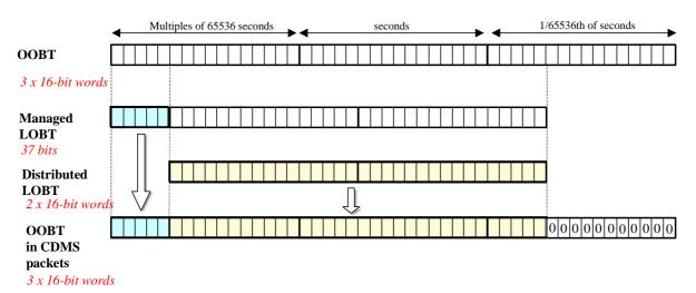
Figure 6 Reconstruction of on board time in CDMS packets
