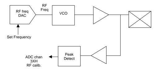
By setting a scan function that produces a constant RF output and stepping the RF frequency DAC whilst reading the resulting RF signal from the RF calibration channel, it is possible to check the calibration of the RF circuit. It is possible that this calibration may drift over the mission lifetime.
