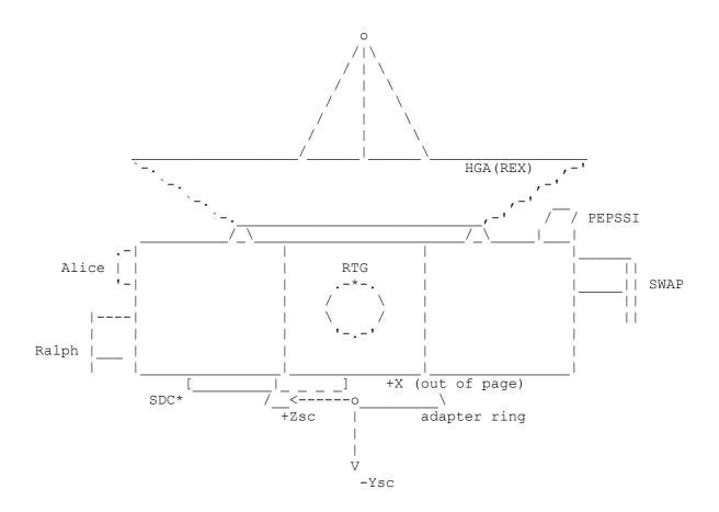
\* N.B. In the graphic above, SDC is behind, i.e. in the -X direction from, the adapter ring
