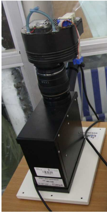
Figure 7.3: The spectrograph unit. The SBIG ST-10ME CCD camera is on top of the CANON objective lens. The object fiber connects to it from the back.
