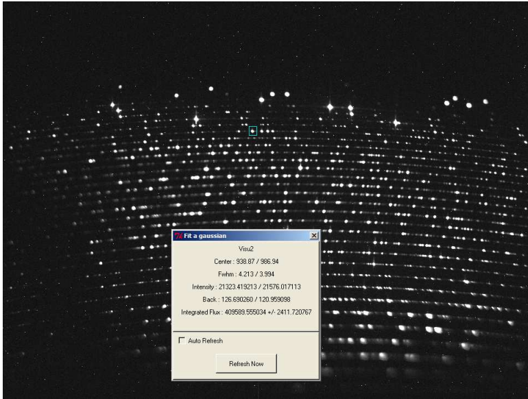
Figure 7.7: Image of the ThAr calibration with the reference line marked and measured with the "Fit a gaussian" analysis function
