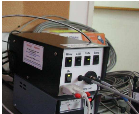
Figure 7.2: The calibration unit with the switches that control the calibration sources and the FIGU mirror
