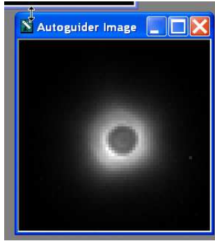
Figure 7.10: Autoguider on a star with the pinhole in the middle.
