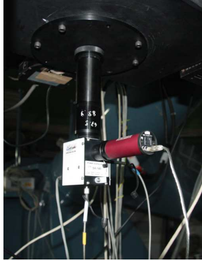
Figure 7.1: The FIGU mounted on the 1m Telescope through a focal reducer
