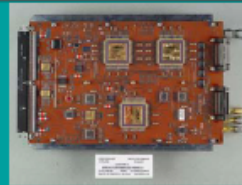
Radio Science Experiment (REX). CBE mass 0.1 kg, power 2.1 W
