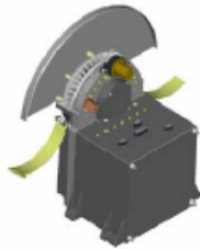
Pluto Energetic Particle Spectrometer Science Investigation (PEPSSI). CBE mass 1.41 kg, power 2.32 W
