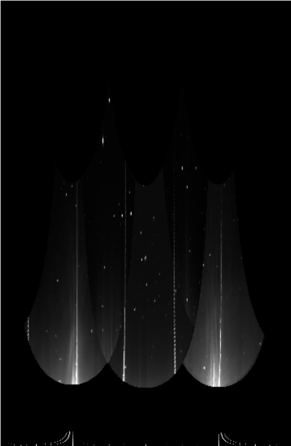
Figure 43 - The same HRI data as in Figure 42 converted to polar coordinates with one degree increments.
