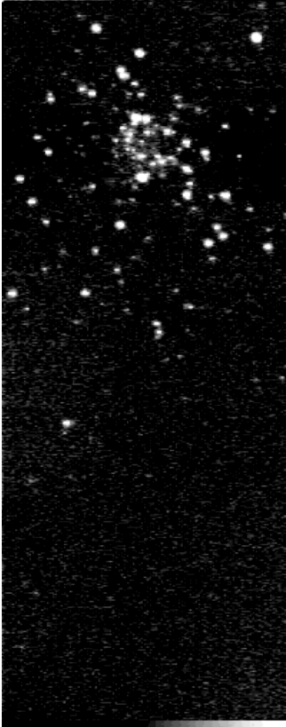
Figure 58 - IR field of view during scan of 47 Tuc. The field of view is one hundred slits wide and 512 physical pixels tall. To have matching spatial scale in both directions, the image has been stretched by a factor of two in the scan direction.
