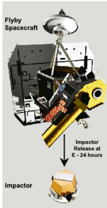
Figure 1. The Deep Impact flyby spacecraft and impactor shown at the time of impactor release, 24 h before the intended impact on comet 9P/Tempel 1.
