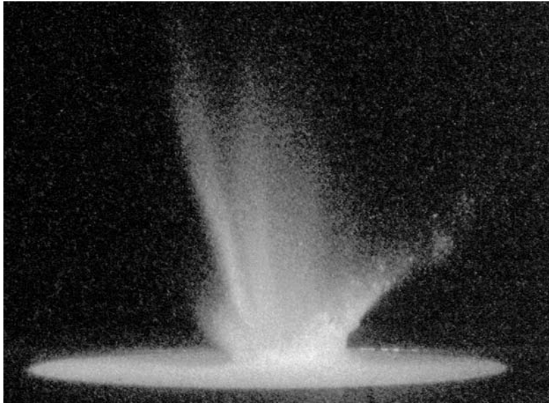
Figure 10. Impact into sieved perlite at 60^\circ (0.318 cm diameter Pyrex sphere at \sim 5.6 \text{ km s}^{-1} ) results in a two-component ejecta plume at late stages: a high-angle plume due to deep penetration and an outward-advancing curtain related to shock rarefaction off the free surface. The high-angle plume gradually evolves as the cavity opens.
