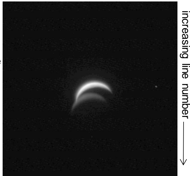
Figure 16 - Doubled image of the Moon taken partially through the periscope at scan mirror angle of 15°; log stretch
